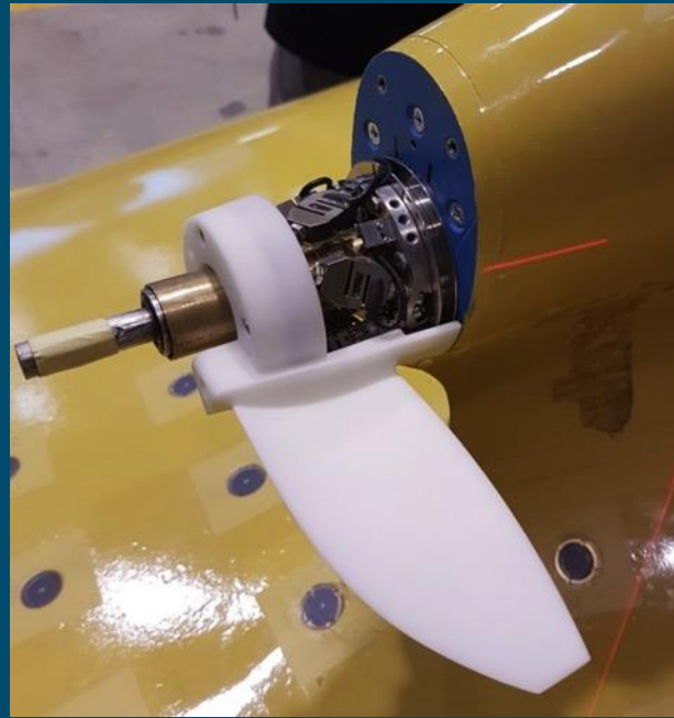
Loads on fins are measured using load sensors
