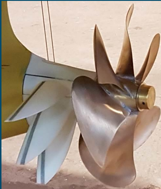
Model propeller and EnergoFlow
