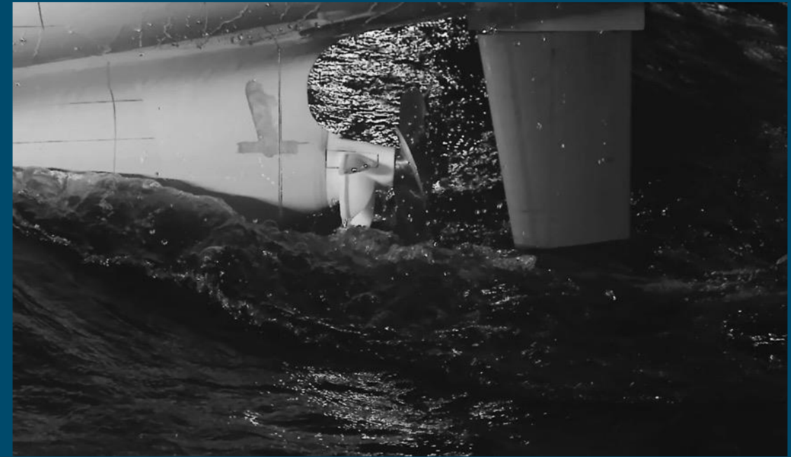
Model-scale seakeeping tests
