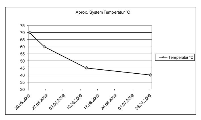
The Viscosity has due to the temperature decrease increased from 13 cSt to 34 cSt. This is accomplished without any increase of the oil's traction properties. This is very positive for the energy consumption and lubrication of all the machine internal components as well as oxidation speed.
