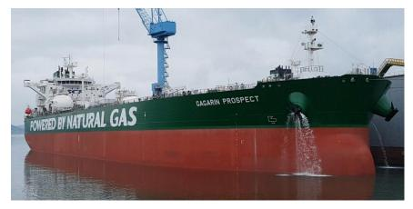
Picture: 7X62DF powered Aframax (Ice class) tanker
