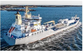
Picture: 5RT-flex50DF powered chemical tanker
