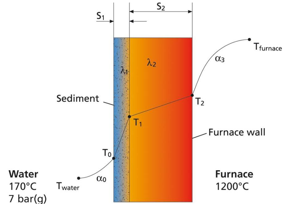
If the waterside of a furnace wall is fouled with e.g. carbonate, silica, or oil film, the temperature of the furnace wall increases due to added thermal resistance.
